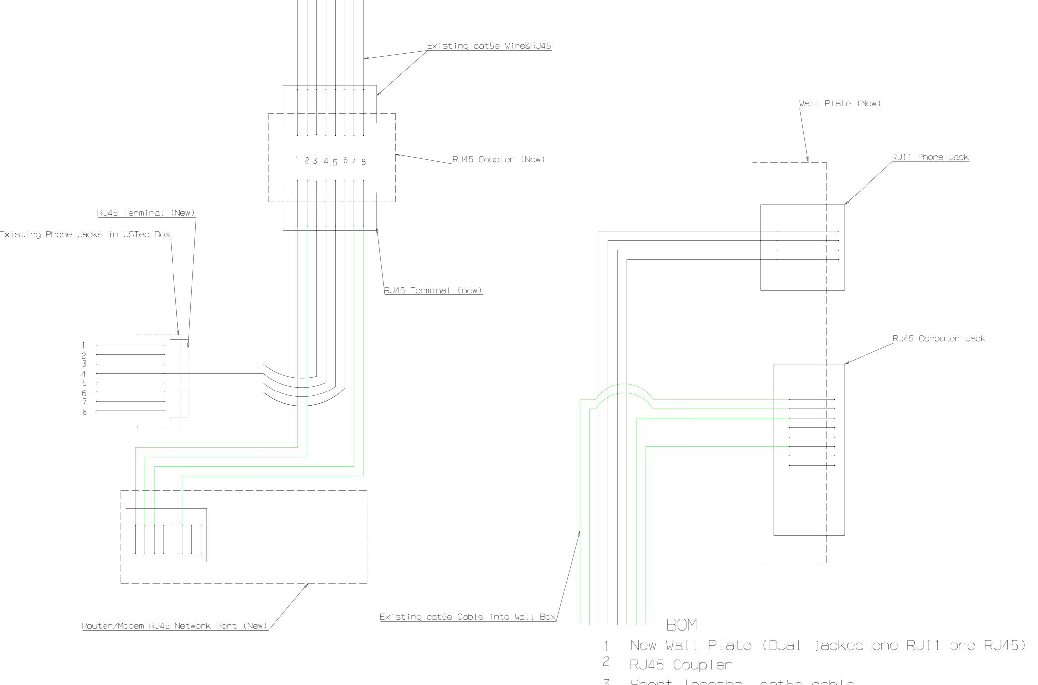
USTec Custom 2-line Phone & Computer Network wiring Utilizing existing 4-line Phone Distribution System
