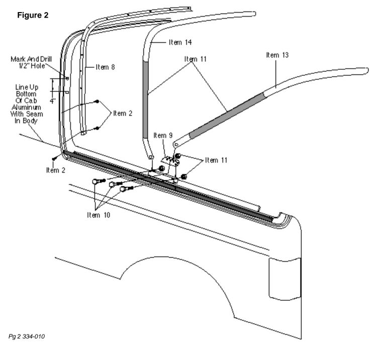
**Step 5. Horizontal Rods.** Measure 4" up from square hole in back of cab. Mark and drill 1/2" hole centered from left to right See figure 2. Place "Top Hat "portion of horizontal rod (Item 15) into this hole and the opposite end into hole in front bow. Repeat for the other side. These rods keep the front bow in position while top is in place.
