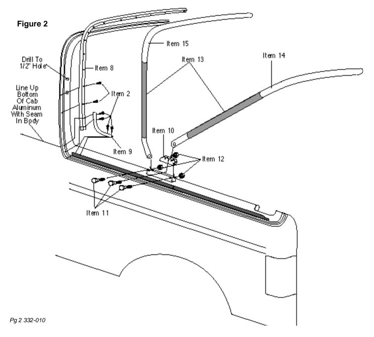
**Step 5. Horizontal Rods.** Measure 3" up from square hole in back of cab. Mark and drill 1/2" hole centered from left to right. See figure 2. Place "Top Hat" portion of horizontal rod (Item 16) into this hole and the opposite end into hole in front bow. Repeat for the other side. These rods keep the front bow in position while top is in place. See figure 3.
