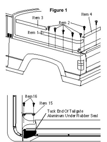
Step 2. Tailgate Aluminum. Mount tailgate aluminum (Item 4) to the top edge of tailgate centered from side to side. Tailgate aluminum should be mounted as far to the rear of flat edge on tailgate as possible. Ends of tailgate aluminum must be placed underneath rubber seal at ends of tailgate. Using tailgate aluminum as a template, mark and drill 1/8" holes. Secure to body with #10 x 1/2" sheet metal screws (Item 2). See figure 1.
